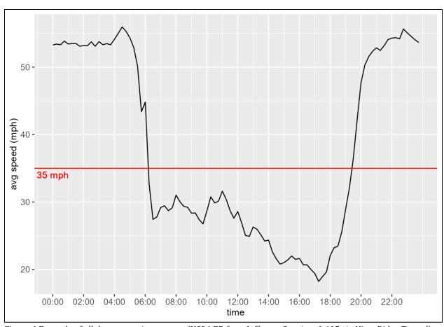
Figure 6 Example of all day congestion pattern (US26 EB from Jefferson St exit to I-405 via Vista Ridge Tunnel)
