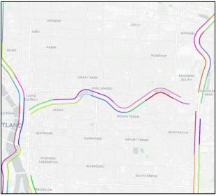
Figure 3 Full throughway segments (left panel) and revised segmentation based on off-ramps (base data: ESRI, RITIS)
