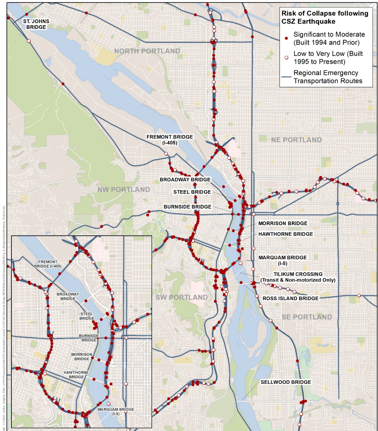
Figure 1.4-2. Risk of Bridge and Overpass Collapse
