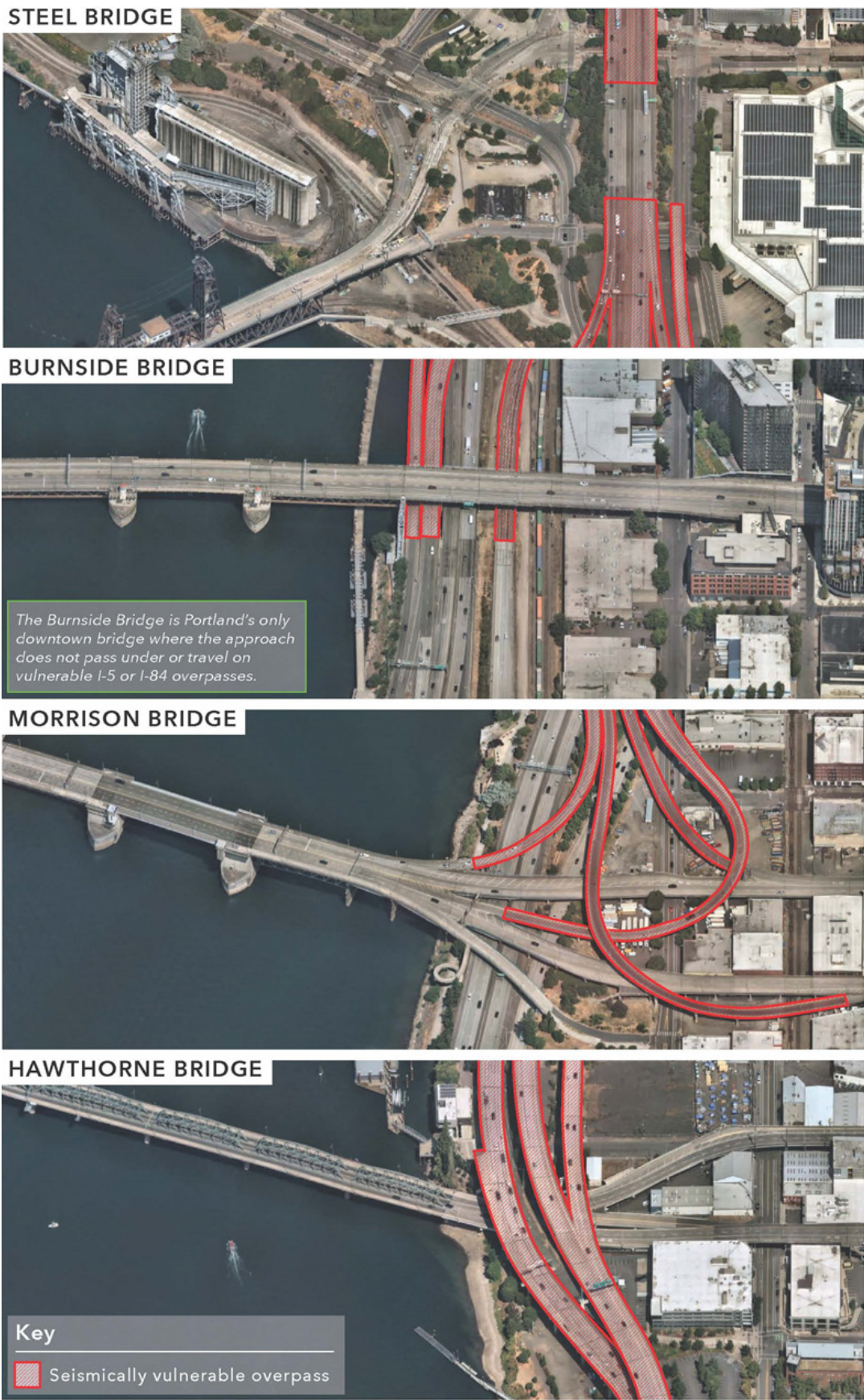
Figure 1.4-3. Seismic Vulnerability of Downtown Bridge Approaches
