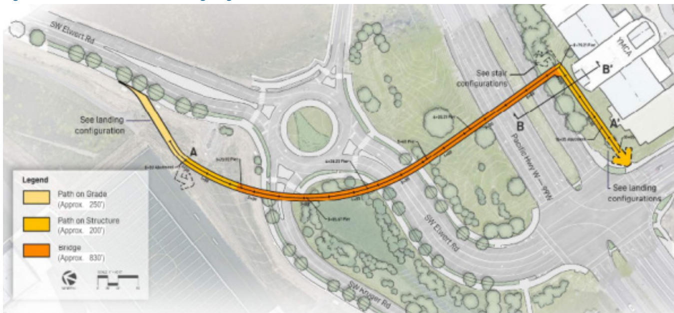
Figure 18. Pedestrian Overcrossing Alignment
