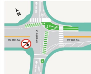
SW 26th Avenue and SW Barbur Court: upgrades include new curb ramps, bike striping and high-visibility crosswalks.
