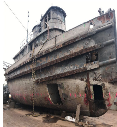
Sakarissa – Sawzall Access Cuts to Hull
