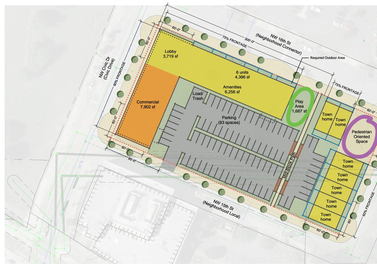
$\label{eq:single_state} \begin{array}{l} \underline{SITE \ DATA} \\ \hline Zoning = CNTH \\ \hline Site \ Area = 83,796 \ sf \ (1.92 \ acres) \\ \hline Building \ Area = 104,072 \ sf \\ \hline Overall \ Floor \ Area \ Ratio \ (F.A.R.) = 1.24 \\ \hline Mixed \ Use \ Density = 82/(30 \ x \ 1.93) + 7,902/(0.9^*83,796) = 1.51 \ (>1) \end{array}$
