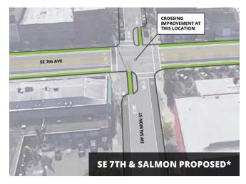
\* Location sketches from 2018 Central City in Motion plan. Proposed project includes concrete traffic separators to protect the bikeway and a center median crossing treatment as SE Salmon
