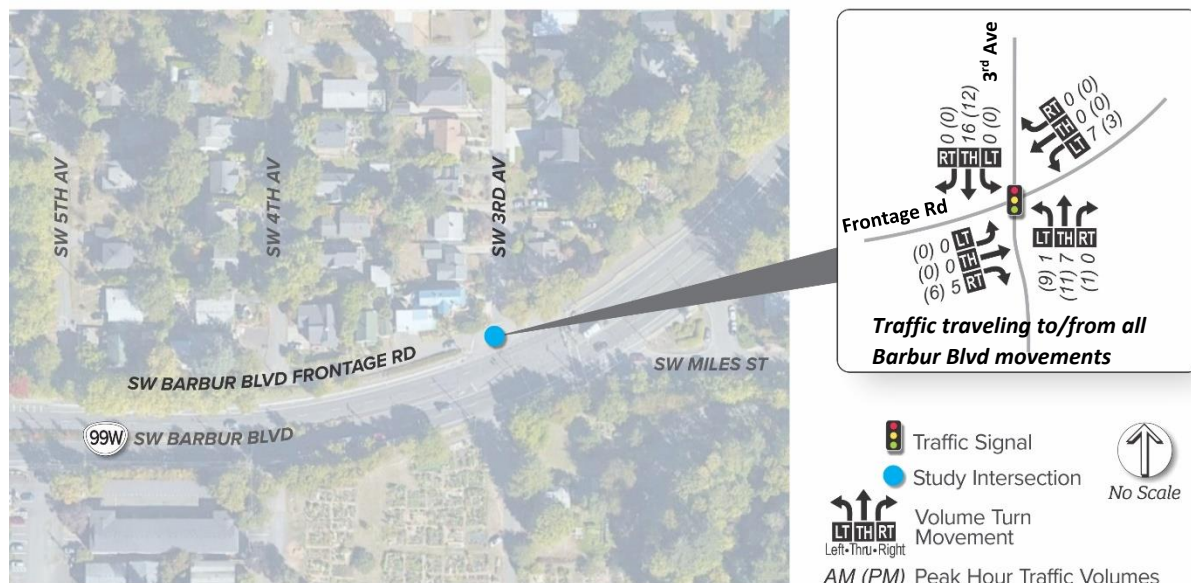
Figure 1: Existing Peak Hour Vehicle Turn Movements at SW 3 rd Avenue/SW Frontage Road
