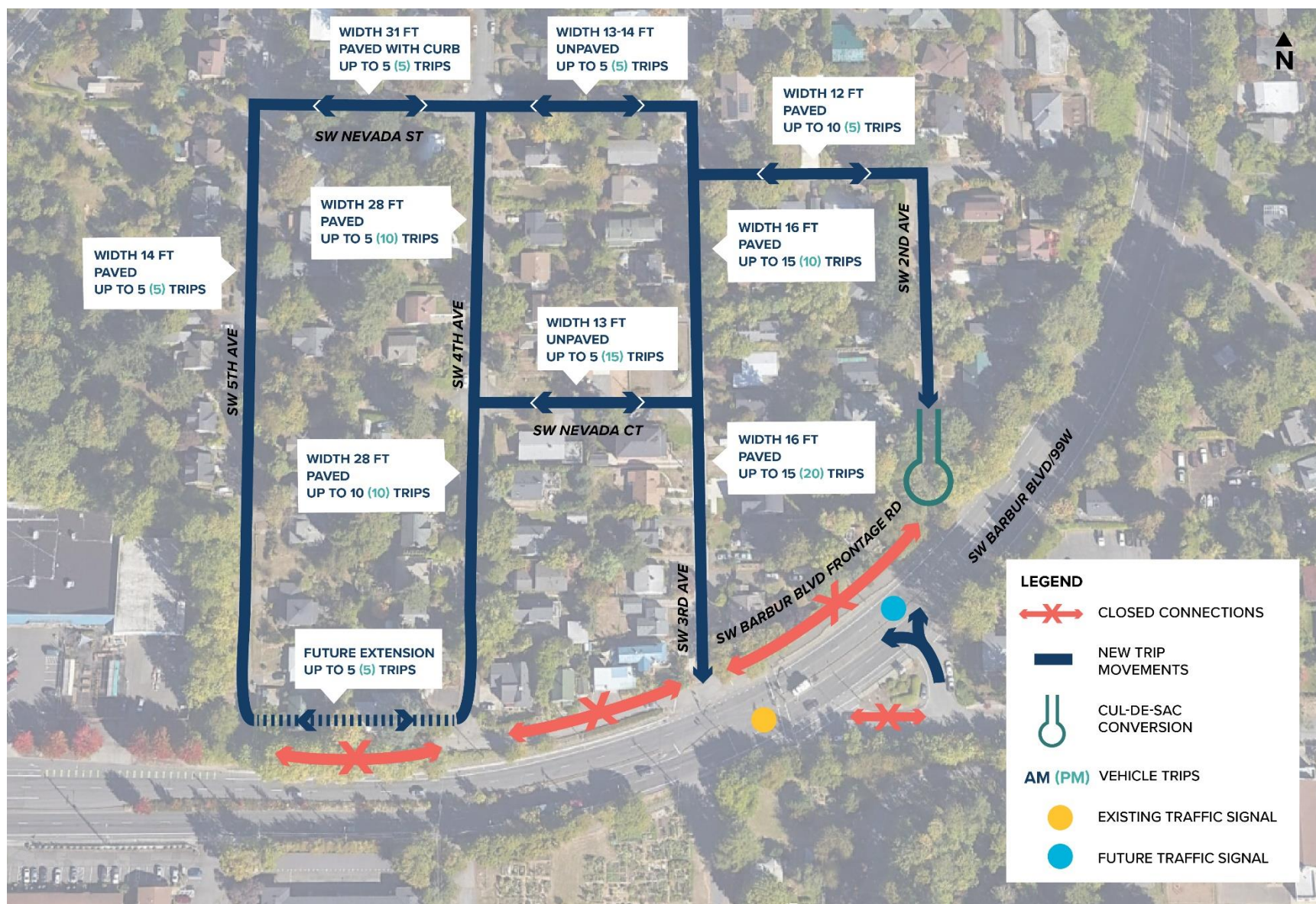
Figure 2: Existing Roadway Characteristics and Added Peak Hour Traffic with LPA Circulation Modifications
