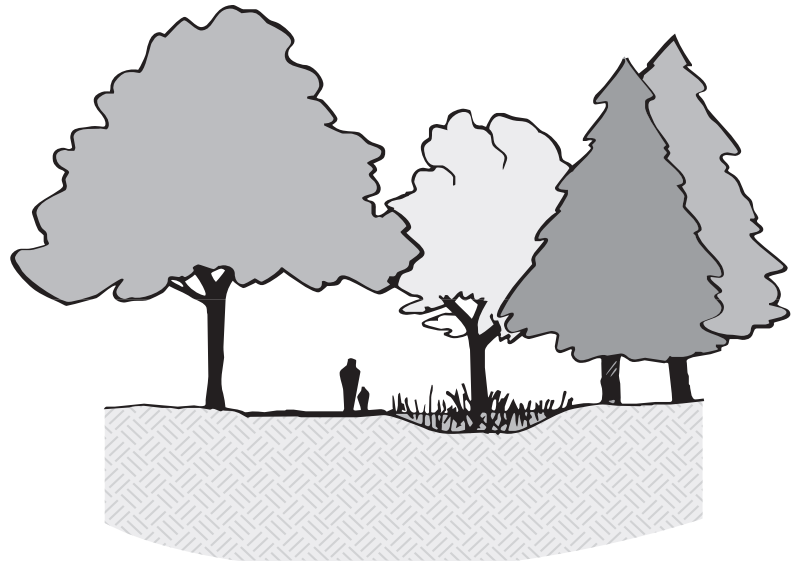
Figure 5-13 Bio-filtering swale. (Green Streets: Innovative Solutions for Stormwater and Stream Crossings, 2002). Vegetation in trailside ditches and swales can slow and filter trail runoff, providing important water resource protection.
