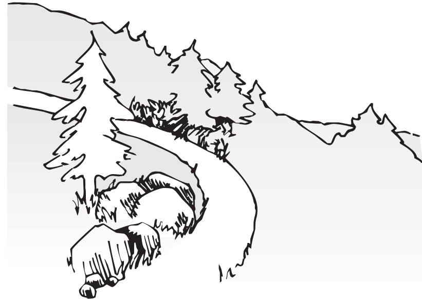
Figure 5-17 Climbing turns sweep gently upslope, minimizing the portion of the trail that runs “with” the slope and keeping gradient low. (Hesselbarth, W. 2000. Trail Construction and Maintenance Notebook. USDA Forest Service.)
