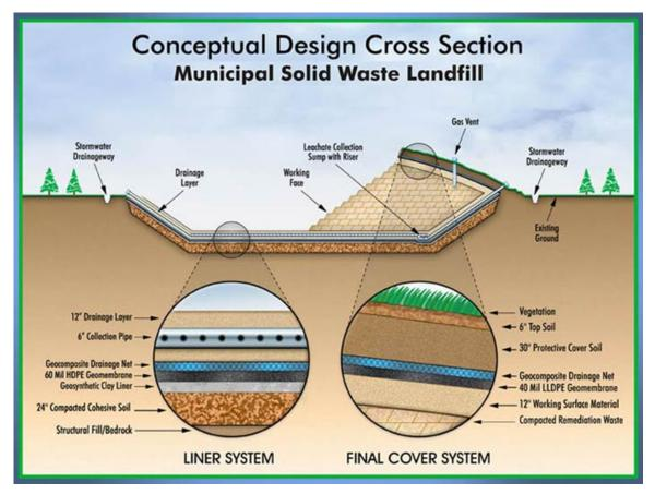
Figure 1. Typical cross section of a modern landfill<sup>4</sup>
