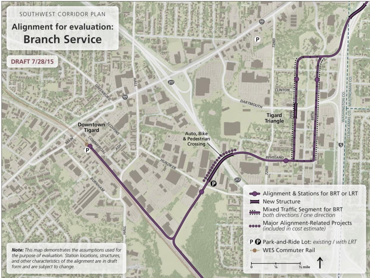
As with the Downtown Loop option, HCT would cross OR-217 on a new bridge between Beveland Street and Wall Street, which would include facilities for cars, bikes, and pedestrians. The alignment would include a station near Hunziker Street and Wall Street. From there, transit vehicles would continue along Wall Street, connecting to the WES corridor; Wall Street would continue to be a dead end street for other modes.
