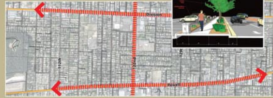
Powell is candidate for a road diet (road narrowing) given its current low traffic volumes (20,000 AADT)
