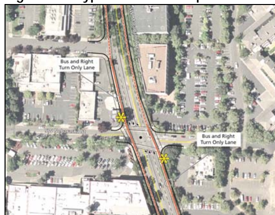
Figure 4-2. Typical Queue Jump
