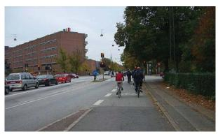
Figure 20. Cycle Track dropping to a marked bike lane at an intersection
