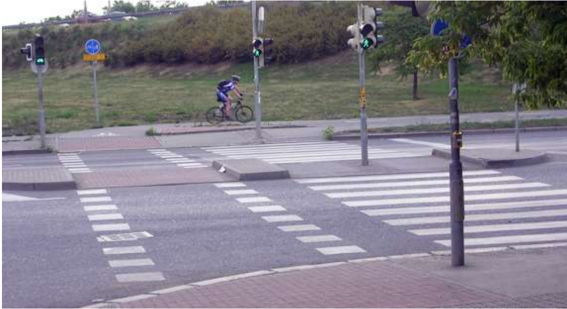
A refuge island provides a protected crossing of an arterial street for pedestrians and bicyclists to access a multi-use path. Photo: Northfield Non-motorized
