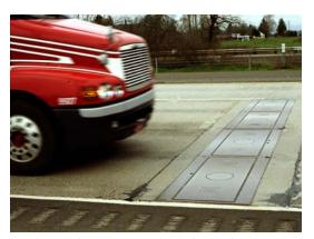
Scales in the pavement weigh trucks as they pass while sensors above check their credentials.
