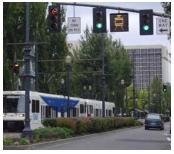
Signal technology at this intersection keeps cars from turning when a train is approaching.
