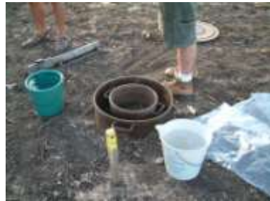
Double Ring Infiltrometer
