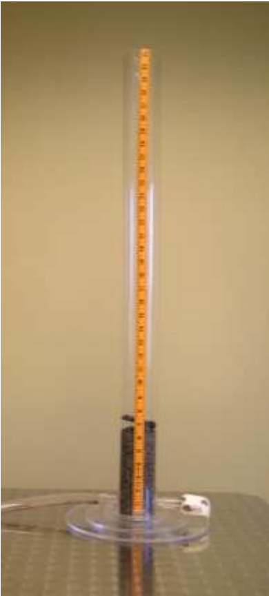
Falling Head Perco-Meter
