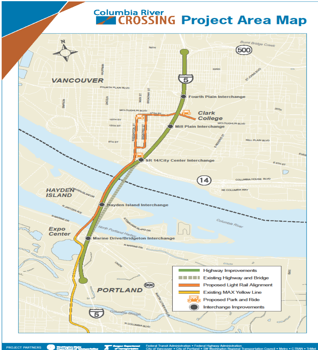
Figure 1: The CRC project replaces a 6 lane bridge with a 10 - 12 lane bridge, LRT and pedestrian/bike facilities and connector improvements.
